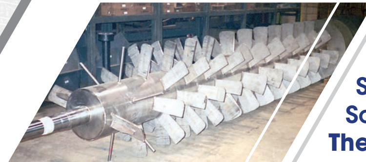
30' long, 48" diameter 316 stainless steel paddle type screw.
