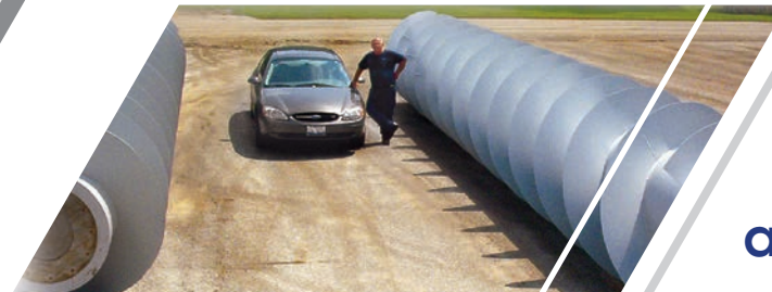
46' long, 78" diameter double lead water lift screws made by Martin .
