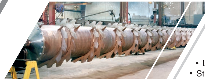
36' long, 38" diameter 2205 duplex SS pulp screw.
